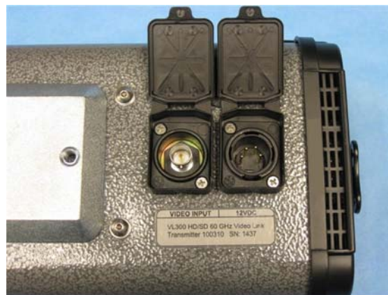
Figure 2. Video and Power Connectors on Bottom of Enclosure
